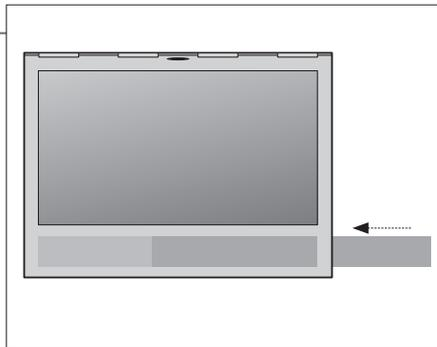
To remove the speaker cover, gently push it out using one of the four pins removed from the television. If the television is mounted on the table stand or wall bracket, you must first remove the sides on the stand or wall bracket to remove the speaker cover. See the guides enclosed with the stand or wall bracket.
